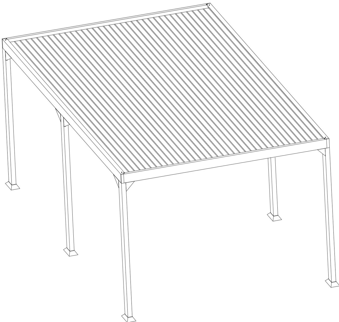
**REMARQUE 1 :** EN DERNIERE ETAPE, VEUILLEZ VOUS ASSUREZ QUE LES RAILS SOIENT TOUS AU MÊME NIVEAU POUR UNE FERMETURE OPTIMALE DES LAMES D'ALUMINIUM. IL EST IMPERATIF QUE LES RAILS SOIENT DROITS ET NON LÉGÈREMENT INCLINÉS.
